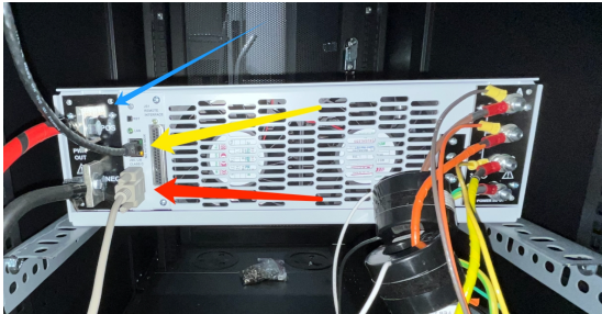
Fig. 6. TDS-1000-15 DC Power Supply Instrumentation and Comms. Wiring
