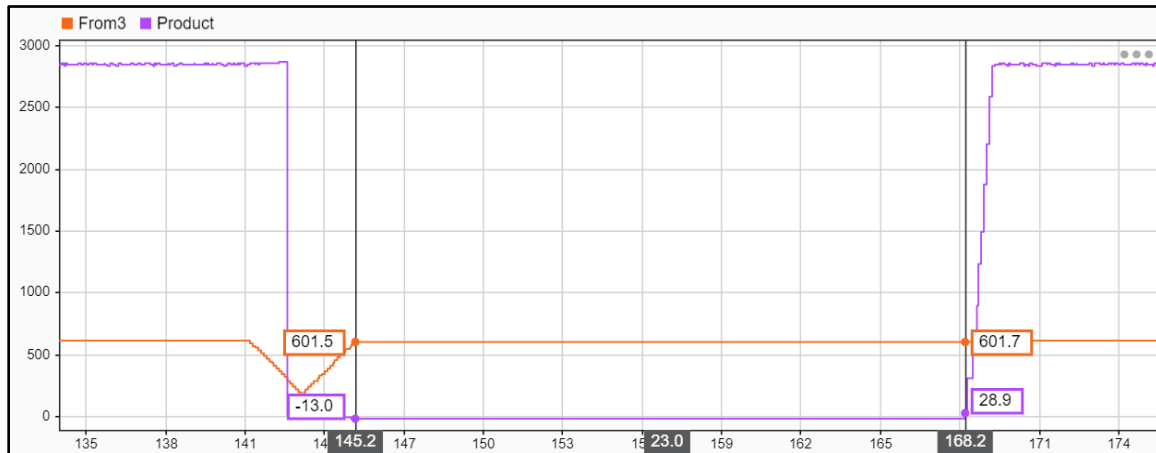
Figure 49 - Return to Service Meter Data Plot (Purple line: Active Power Orange Line: Voltage)
